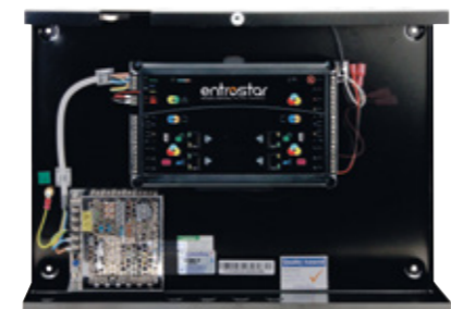
EntroStar in a metal enclosure with a PSU (optional battery)
